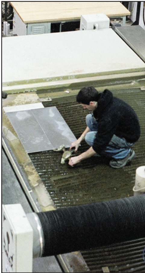
Right: On top of the machine, Dery securely clamps two sheets of steel in place before they are submerged and sawed through.
