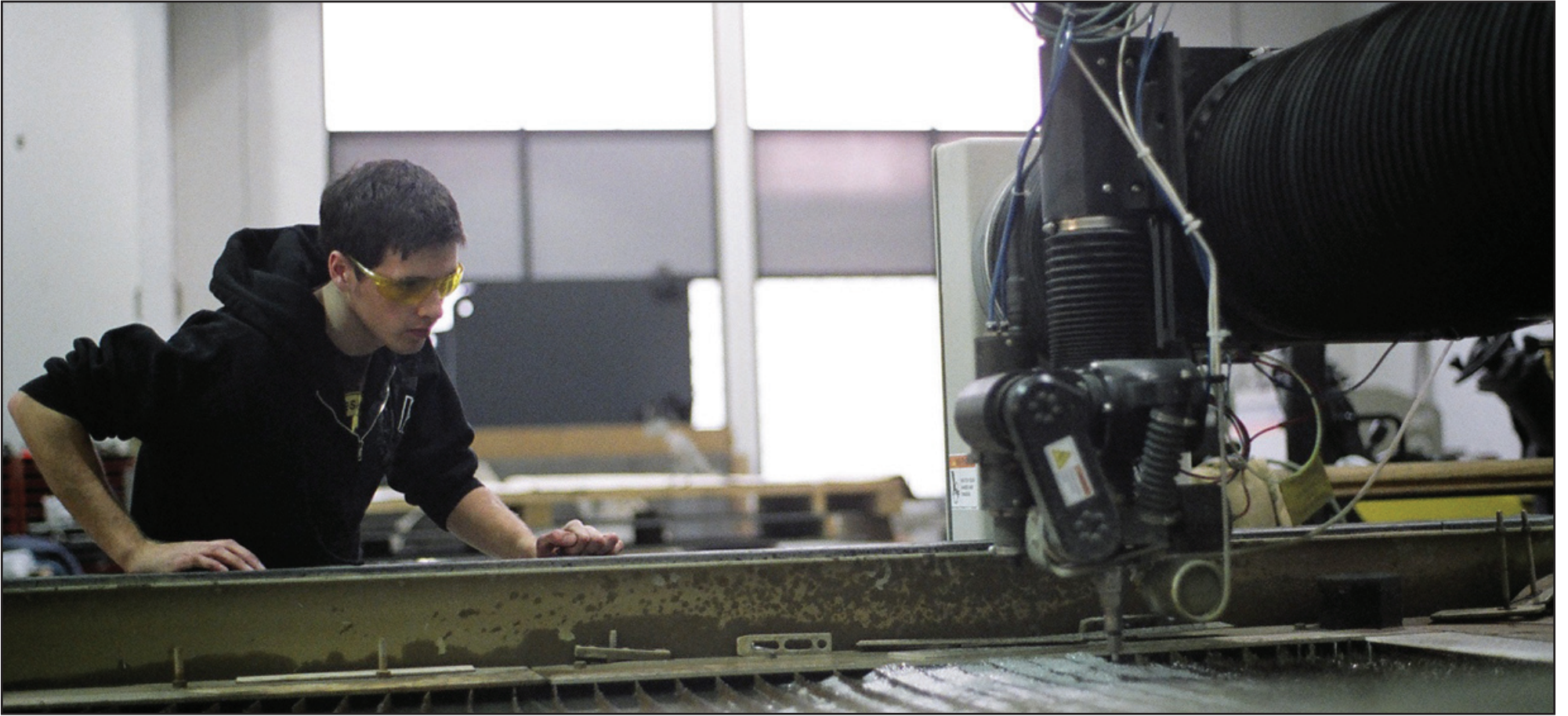
Jordan Dery, a machinist, monitors the progress of the Omax high pressure waterjet machine as it cuts through steel underwater at Karice Enterprises in Surrey on Friday afternoon. The machine uses a mixture of water and fine sand to cut through metal, stone, wood and glass.
