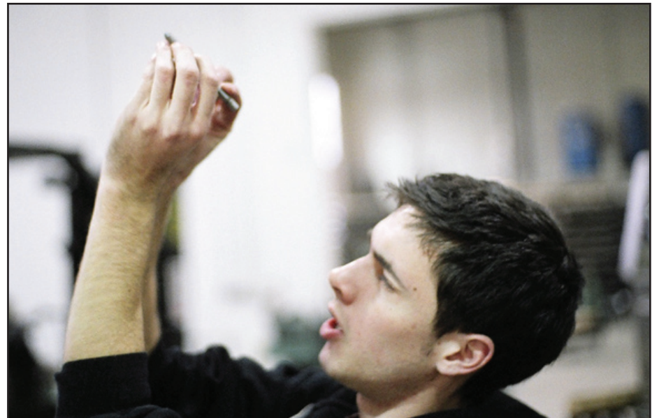
Below: Dery checks for damages on a mixing tube, the part of the machine where the water mixes with the sand.
