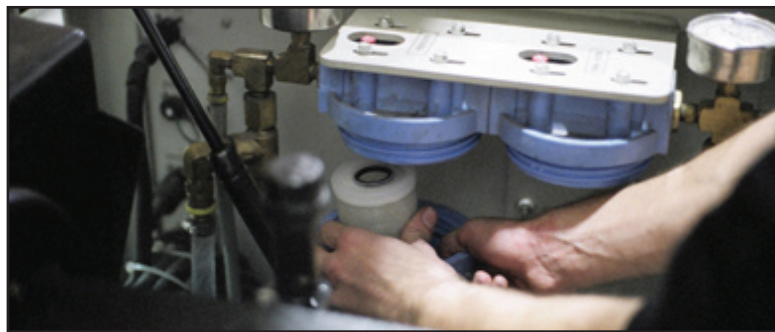
Below: Dery checks for damages on a mixing tube, the part of the machine where the water mixes with the sand.
